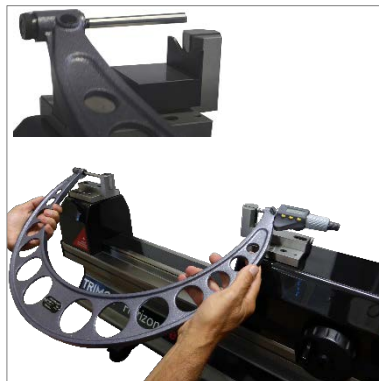
Manually checking of external micrometer (TEL5)
