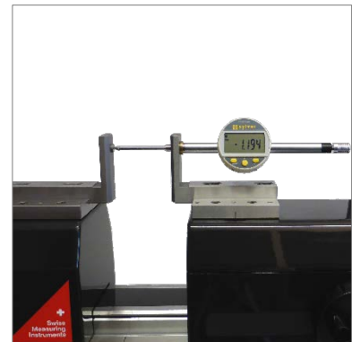
Checking of dial indicator (TEL5CN)
